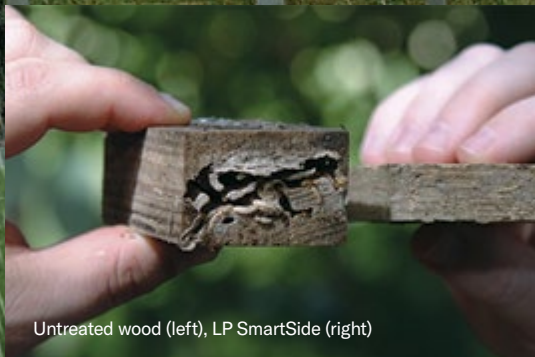
LP SmartSide product testing in Hilo, Hawaii
