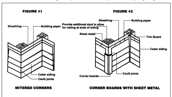
overlapping joint. Butt joints between boards should be staggered and made on studs. Caulking butt joints is recommended.
